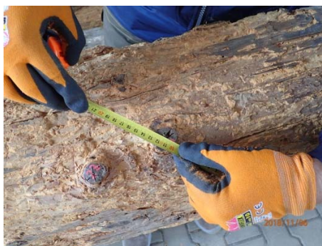
Figure 3: measurement of knot dimensions and position along the member
